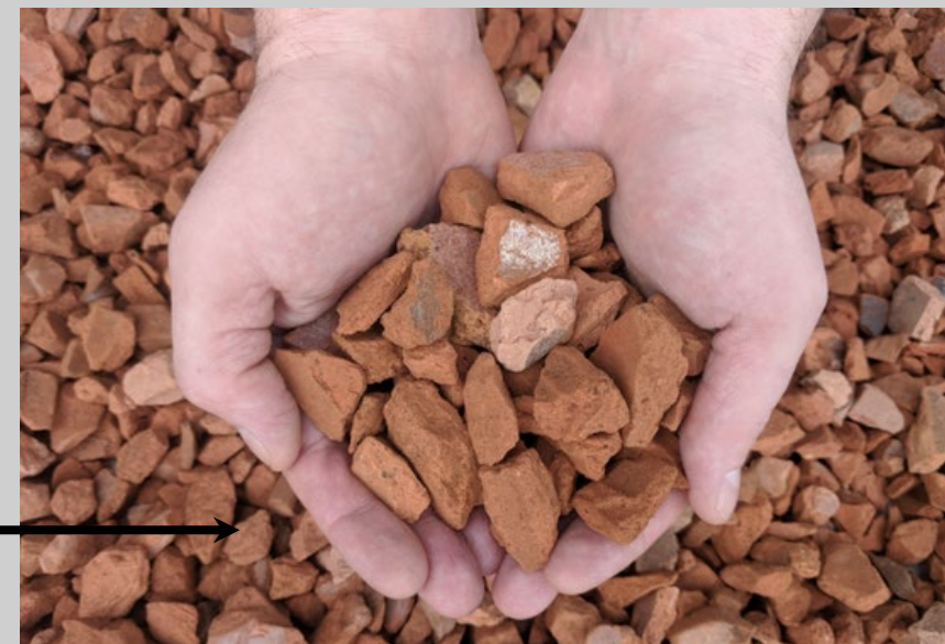
crushed roof tiles to be recycled.
