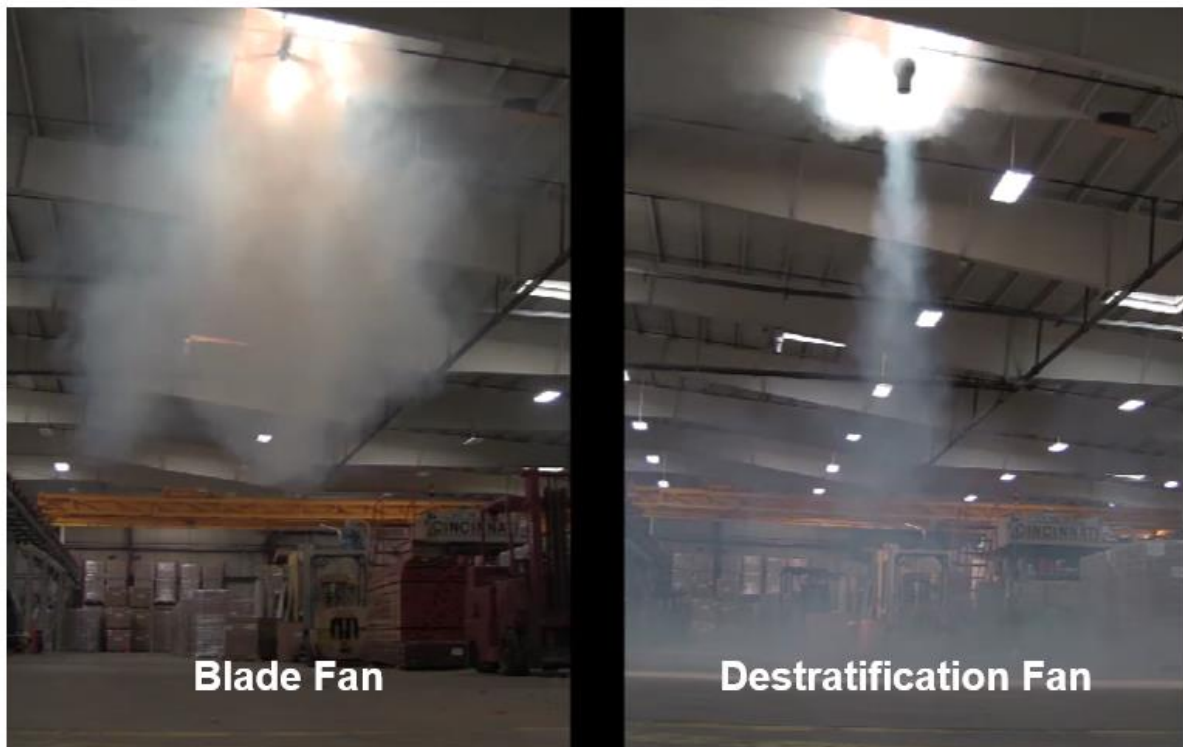
Figure 19: Smoke Test Showing Airflow of Destratification Fan
