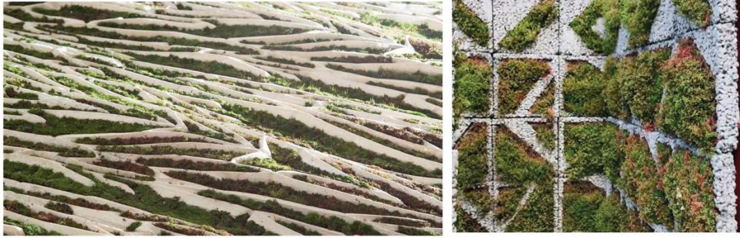
Figure 29 Results of experiments from Professor Marcos Cruz and lecturer Richard Beckett in Bartlett School of Architecture at University College London. Which they have been researching how concrete can be made more bioreceptive, and have developed facade panels specially designed to encourage the growth of cryptogams.
