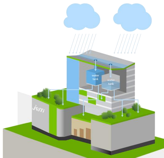
Figure 31: Rainwater Harvesting System (Jem, Rainwater harvesting system)
