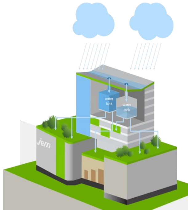
Figure 46: Rainwater Harvesting System at JEM Shopping Mall
