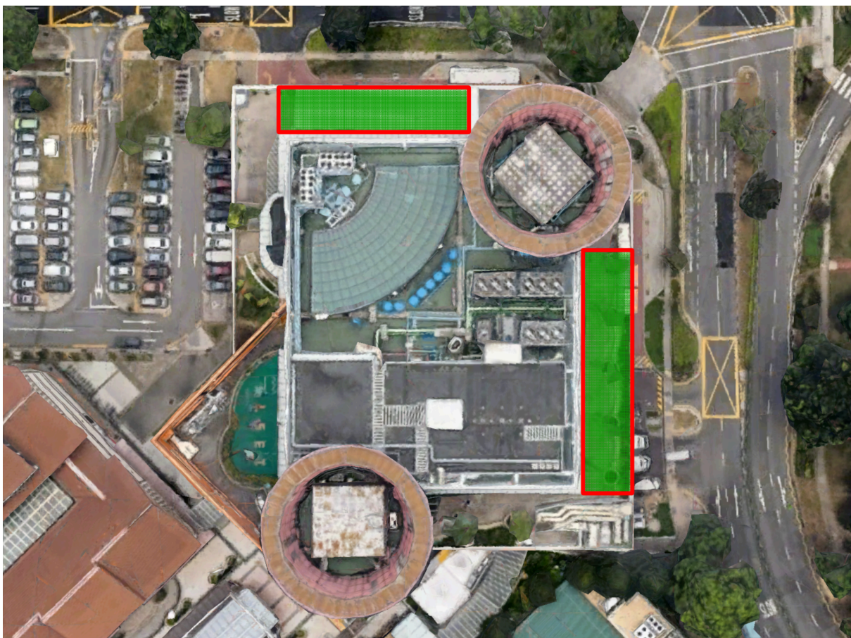
Figure 8: Placement of rainwater harvesters on rooftop
